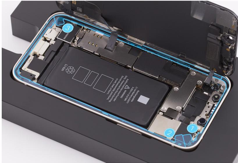
20. Inspect the display adhesive to ensure that it's in the correct position and not damaged or wrinkled. If the adhesive is damaged, remove it and apply replacement adhesive.
