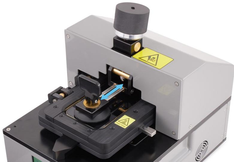
9. Turn the knob on the fixture clockwise to lower the suction cup onto the display (1). Then flip down the handle on the suction cup to secure the suction cup to the display (2).
