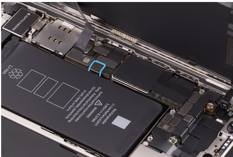
26. Use the black stick to lift the ends of the display flex cable (1) and the receiver flex cable (2) off the connectors.
