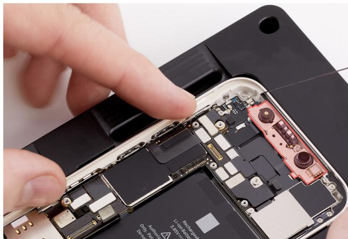
30. Use ethanol wipes or IPA wipes to clean any adhesive residue from the enclosure.
