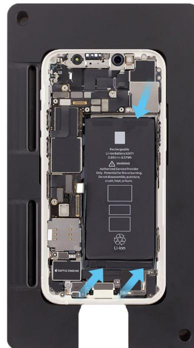
14. Slightly lift the battery with the black stick just enough to grasp underneath the battery.
