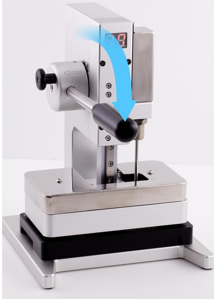
26. Wait until the timer on the display press beeps. Pull down the lever (1) and pull out the release knob (2). Then lift the lever (3).
