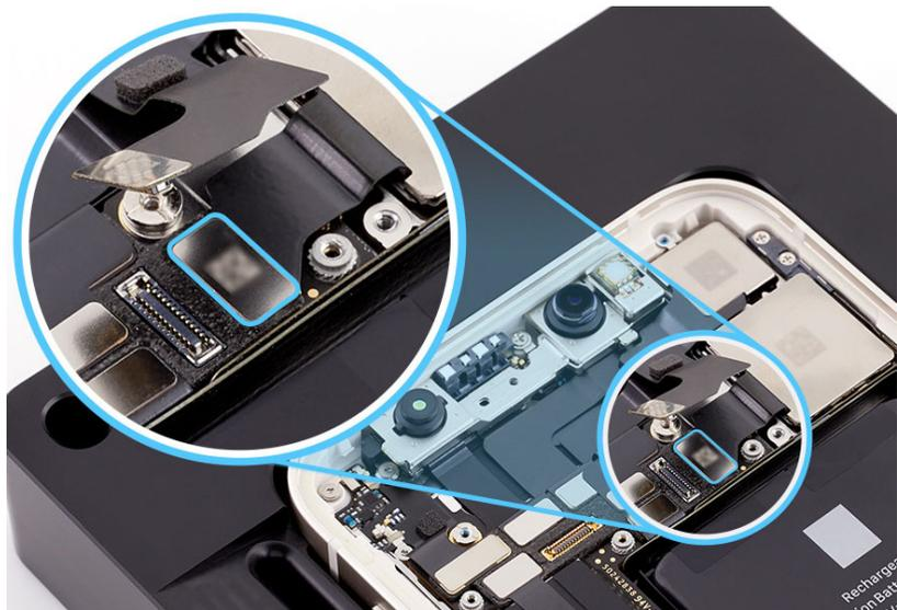
4. Press the end of the top camera flex cable to the connector.
