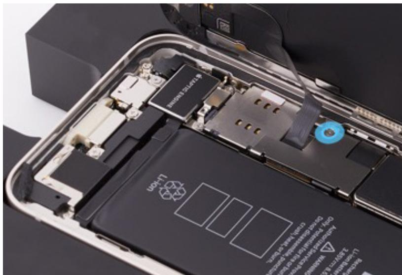
22. Use ESD-safe tweezers to remove the lower cowling. Save the cowling for reassembly.
