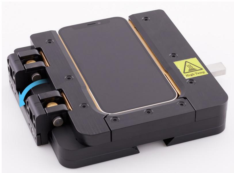
5. Put on the heat-resistant gloves. Align the cutout on the bottom of the pocket with the rail on the fixture. Slide the pocket with the iPhone onto the rail on the fixture.
