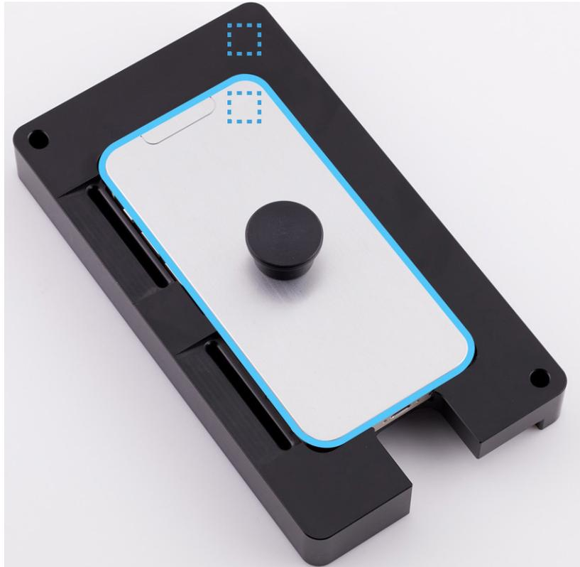
7. Position the repair tray with the iPhone in the display press. Pull down the lever until the display press locks.
