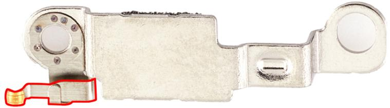
6. Use the green torque driver and JCIS bit to install two new crosshead screws into the Taptic Engine connector cowling.
