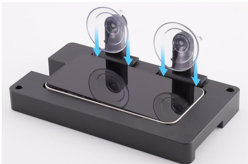
20. Tilt up the display toward the suction cups. Press the top and bottom edges of the display to secure it to the suction cups.
