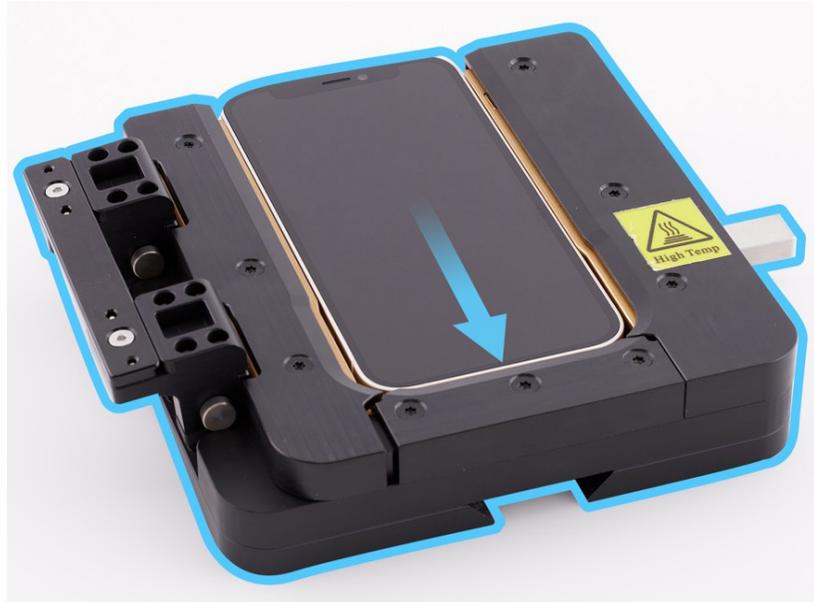
4. Flip down the clamp on the side of the pocket to lock the iPhone into place.
