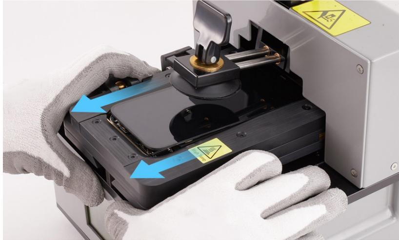
15. Flip up the clamp on the side of the pocket to release the iPhone (1). Hold the area outlined in blue and gently remove the iPhone from the pocket (2).
