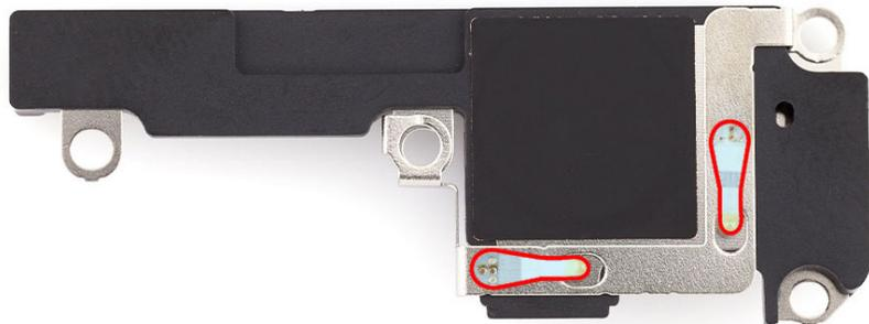
3. Rotate the repair tray. Use the green torque driver and JCIS bit to install four new crosshead screws into the speaker.
