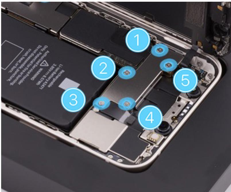
24. Use ESD-safe tweezers to remove the upper cowling. Save the cowling for reassembly.
